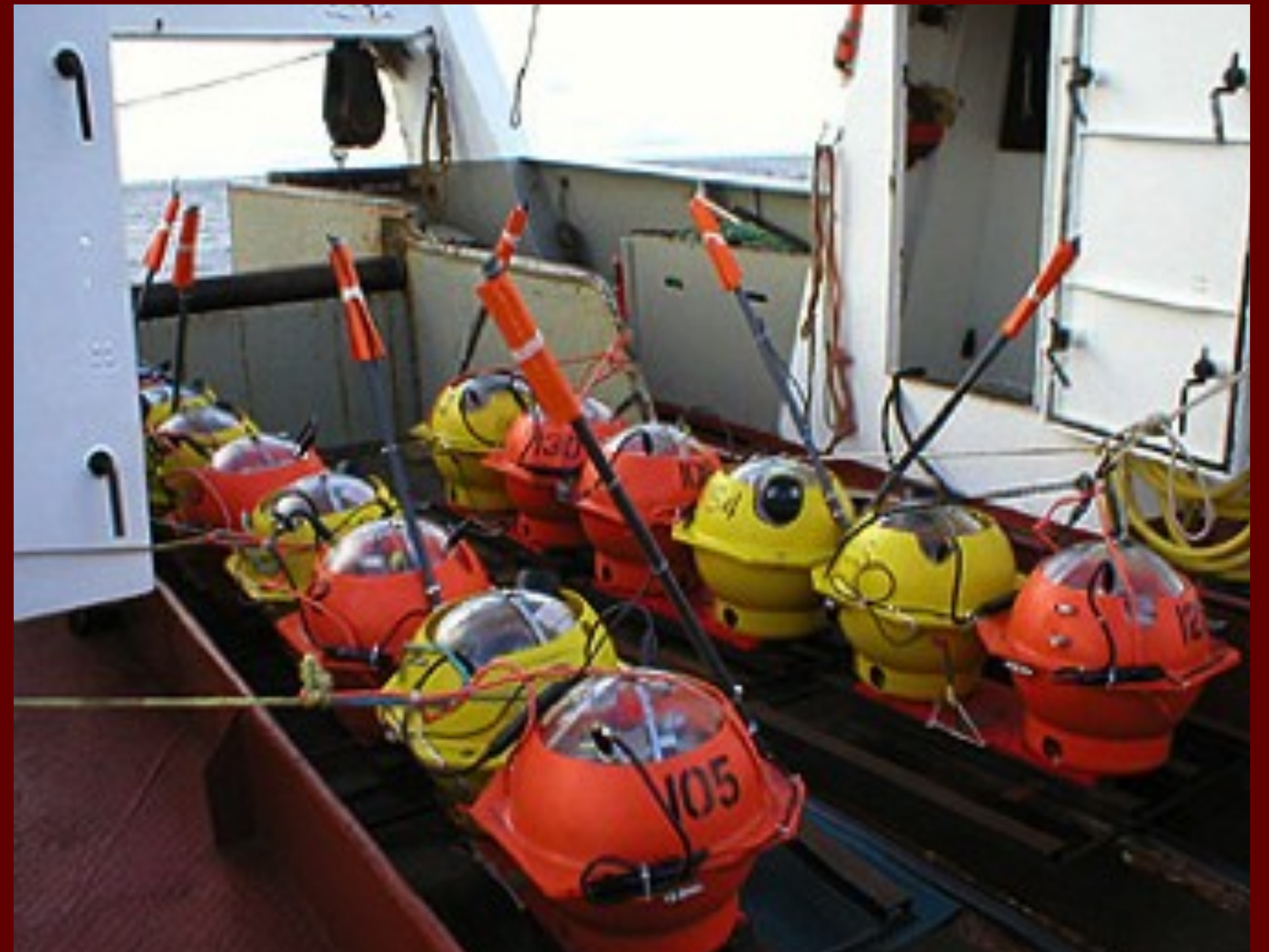
Ocean bottom nodes on a ship
